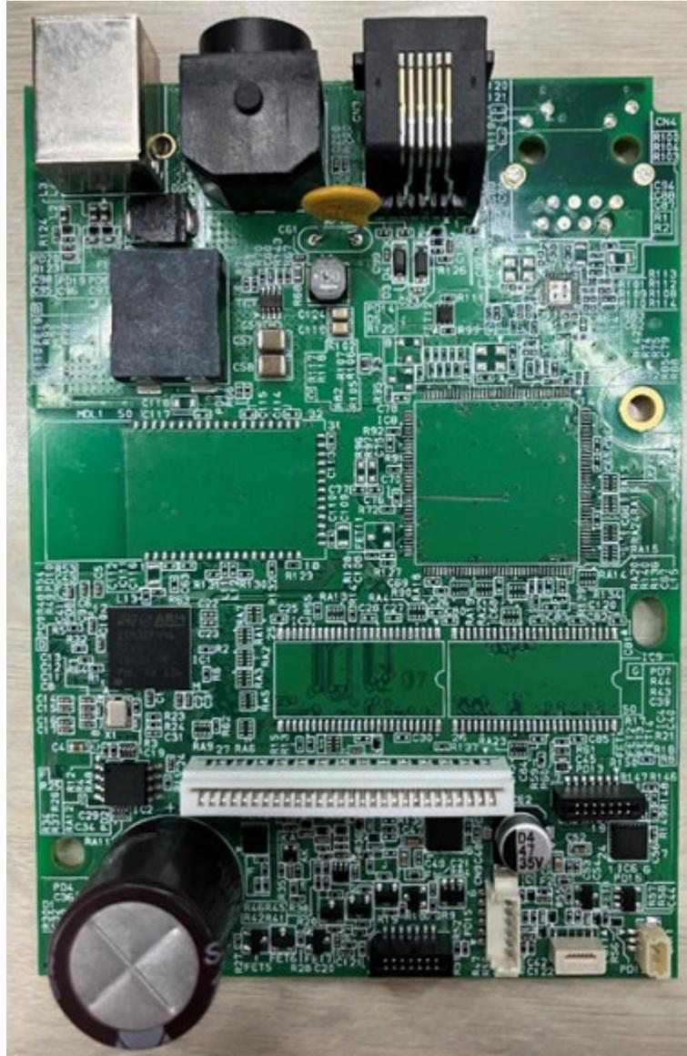
Figure 2-26 Component Layout of Circuit Board (Japan Only) (SLP721RT-U MAIN PCB BLOCK A) (Reference)
