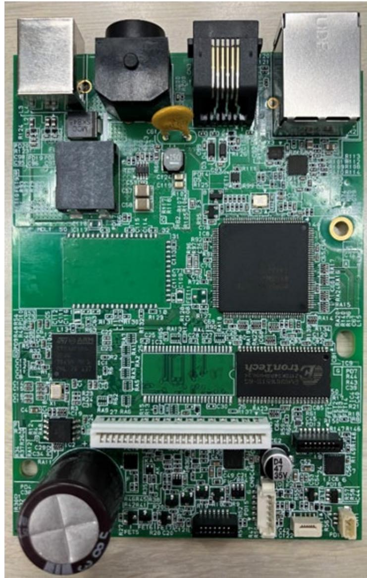
Figure 2-27 Component Layout of Circuit Board (SLP721RT-E MAIN PCB BLOCK A) (Reference)
